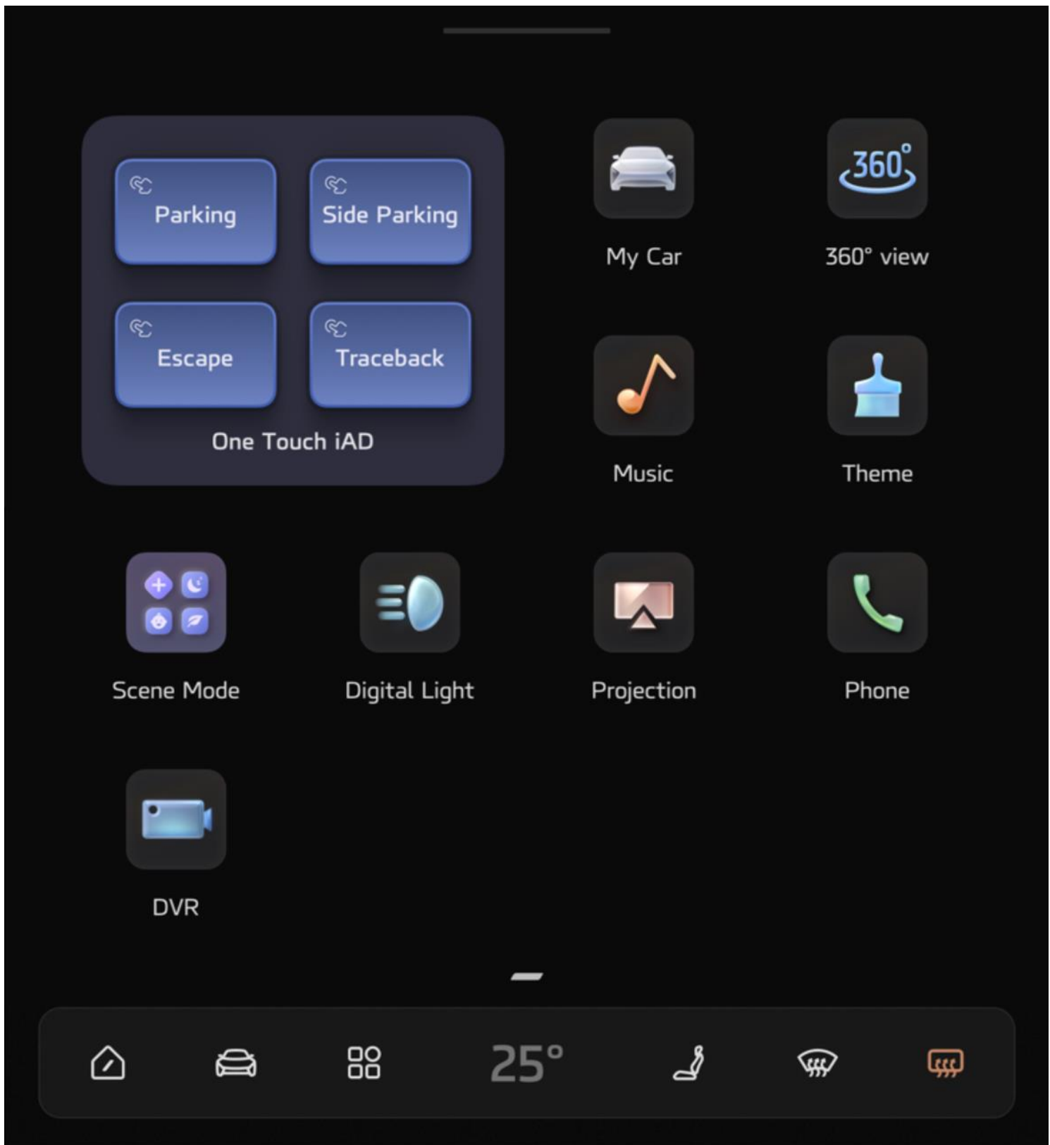
Method 4: Click the “Parking” button on the 360 interface to quickly enable and go to the APA interface.
